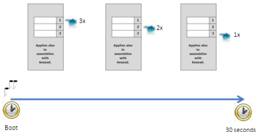
Figure 3.1 Switching to Default Network Parameters – Static IP Address (Order Nos. 9137130E, 9137130CE, 9137130CKE, 9137131E, 9137131CE, 9137131CKE)
